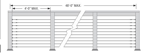
For straight cable sections using the RailEasy<sup>TM</sup> Tensioner at each end, you may run cable up to 48 feet in total length (mid post required as specified).
