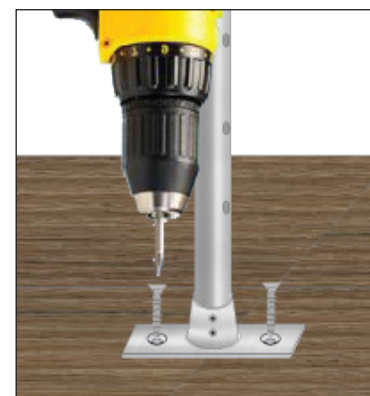
Figure Z. (LEFT) Attach the top of the stabilizer to the underside of the top rail with (2) two 1/4 x 2" flat head wood screws. Figure AA. (RIGHT) Attach the bottom of the stabilizer to the mounting surface with (2) two 1/4 x 2" flat head wood screws.
