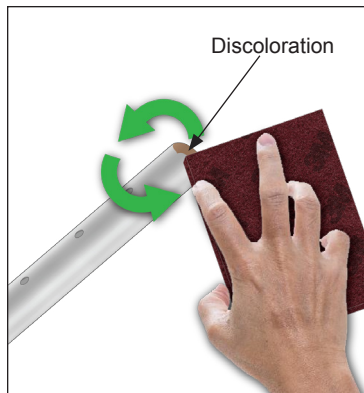
Figure T. (LEFT) Remove any surface discoloration with a Scotch-Brite Pad. Figure U. (RIGHT) Assemble the Cable Stabilizer Kit by re-attaching both the upper and lower stabilizer bases to the stanchion.
