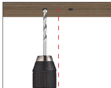
Figure X. (LEFT) Drill pilot holes at the pencil marks in the bottom side of the handrail. Figure Y. (RIGHT) Drill pilot holes at the pencil marks in the mounting surface.
