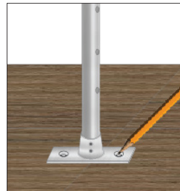
Figure V. (LEFT) Mark screw holes in the upper stabilizer base with a pencil. Figure W. (RIGHT) Mark screw holes in the lower stabilizer base with a pencil.
