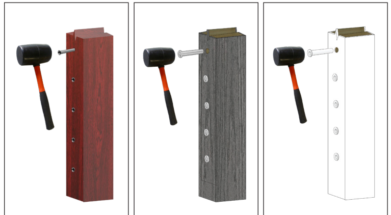
Figure C. Tap Cable Sleeves snugly into place (wood mid post [LEFT], composite mid post [CENTER] and vinyl sleeve post [RIGHT]).
