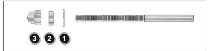
Figure AF. Acorn Nut Set Assembly Diagram - 1) Stainless Steel Washer, 2) Stainless Steel Nut & 3) Stainless Steel Acorn Nut. HandiSwage Stud not included.
