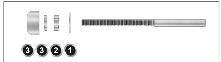
Figure AG Deluxe Cover Nut Set Assembly Diagram - 1) Stainless Steel Washer, 2) Stainless Steel Nut 3) Stainless Steel Lock Nut & 4) Stainless Steel Deluxe Cover. HandiSwage Stud not included.
